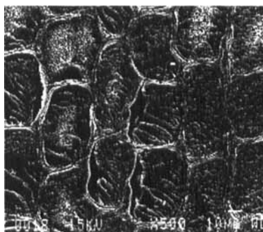
FIGURE 2 Adhesion of polymer to cell walls in WPC made with HDDA and HEMA.
